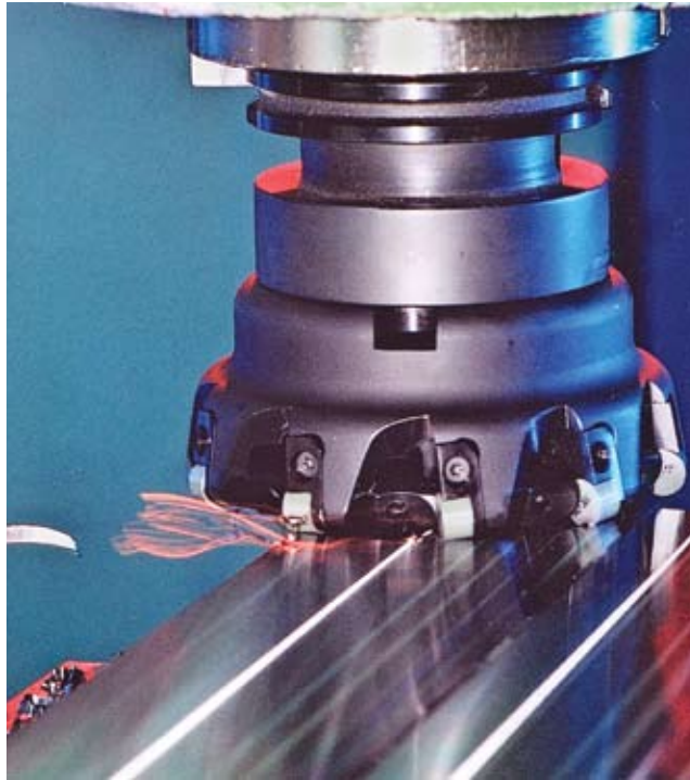
Milling with ceramics can enable a shop to cut machining time and reduce the number of operations required to complete a hard (45 HRC and higher) part.
