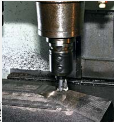
This pyramid-shaped part is one of four hammers used to forge titanium alloys.
