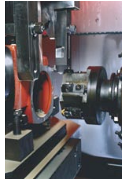
A Greenleaf multifunction cutter poised to machine multiple features on a cast iron housing.
