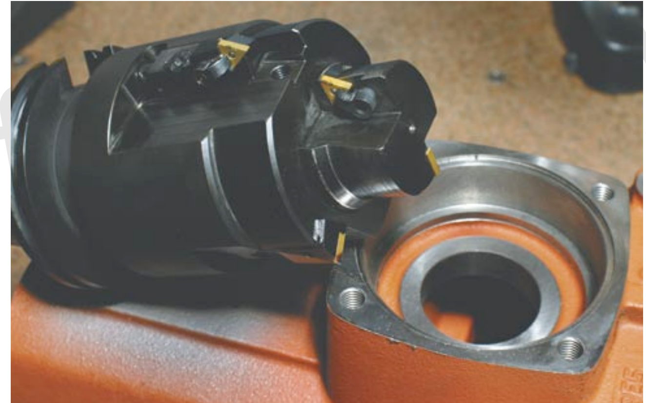
Multifunction cutter and the cast iron housing it was designed to produce.
