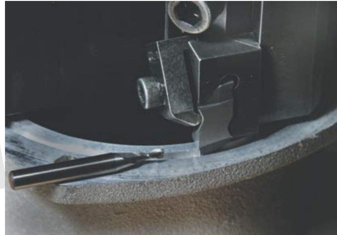
A grooving insert fitted in a multifunction cutter replaced a 2.5mm-dia. endmill that required two passes to interpolate a 2.8mm-wide groove around an aluminum flange face.
