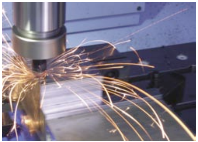
As the ceramic inserts mill the pocket, the heat that is generated by the operation is transferred to the chip, not the part.
